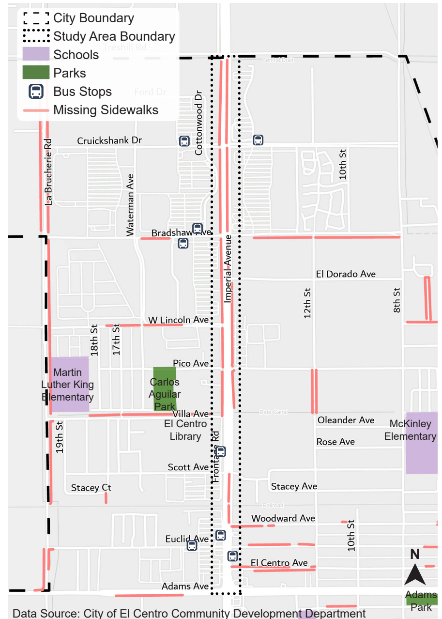
Figure 2-4: Missing Sidewalks on Imperial Avenue
